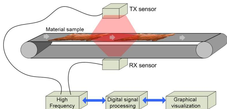
The core of a Wavetester is an innovative microwave measurement principle. Its particularity is in the fact that, in contrast to the other existing systems, the entire thickness of the material is analyzed due to a double antenna system.
