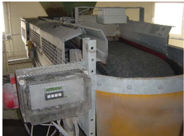
The sensor installed on a concrete mixer
