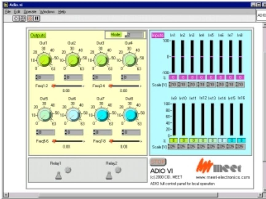
Fig. 2 ADIO virtual instrument user interface (LabVIEW)
