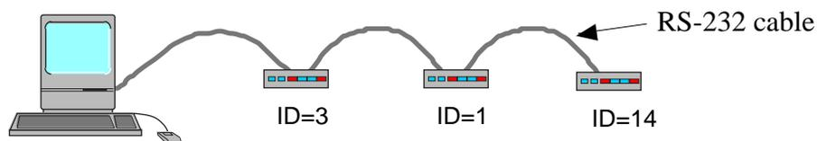
Each ADIO-01 acts as a repeater (with zero delay!) for the downlink modules. This insures a reliable and interference free communication.
